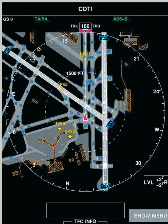
This Surface Area Movement Management (SAMM) display from ACSS gives UPS freighter pilots a view of all the company's cargo jets operating at Louisville's Standiford Field.
