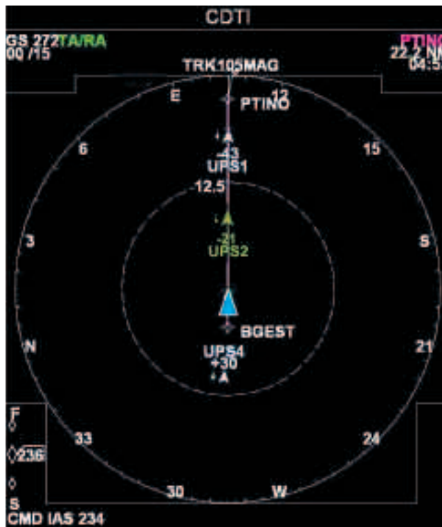
The ACSS merging and spacing software will enable UPS aircraft to fly continuous-descent approaches to Louisville. Blue triangle shows "own-ship" merged behind UPS 2, which is following UPS 1. The pilot uses the speed command (234 kt. IAS) and fast/slow cues (both lower left) to maintain proper spacing. UPS 4 is last in line.
